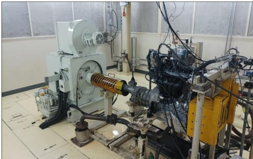
Figure 2. Engine Dynamometer Installation
