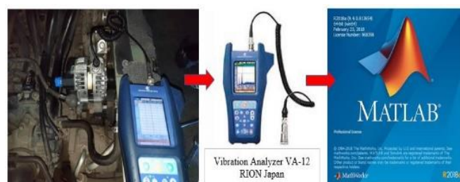
Figure 3. Set-up vibration measurement
